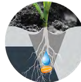
3 SMART FIRMER OR KEETON LOW STICK SEED FIRMER: LIQUID FERTILIZER OR LIQUID INOCULANTS PLACEMENT ON TOP OF SEED
