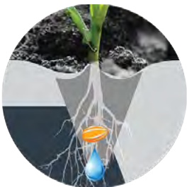
4 SEED BOOT LIQUIDS TUBE: LIQUID FERTILIZER OR INOCULANTS UNDER SEED
